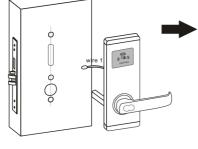
Connect wire 1, Get the handle spindle to go through the relative hole on the mortise and get the front lock body to be close to the door face.
