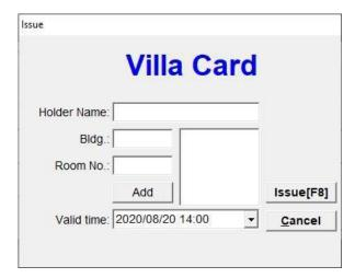
Fill the fields and add a maximum of 6 rooms into the field as needed then click "Issue". It will show "Write Card OK!" if the operation is successful. Click "OK" to finish issuing. You can click the drop down menu and select the "Date Limit" to set the valid time of the card.
