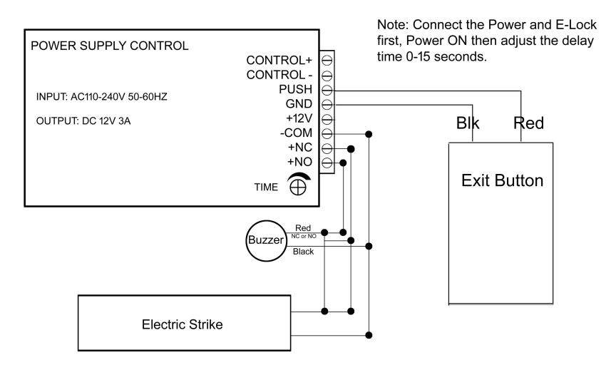
Note: If your Electric Strike is Fail Safe please connect to NC. If it is Fail Secure connect to NO.
