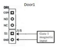
Connect the door sensor to the "S1" and "GND" of the access control board. If you want to use the sensor for door2, simply connect the sensor to "S2" and "GND" of the board, etc.
