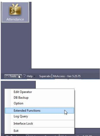
Now we open the access control software. Click on Tools on the bottom left of the software. And then click on the "Extended Functions."
