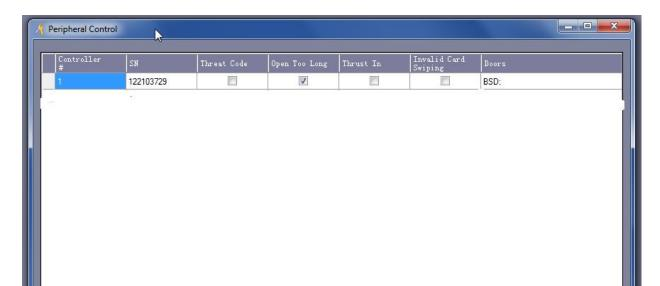
Check the "Open Too Long," and change the "Allowable Open Time," this is the time you allow the door to open without the alarm ringing.
