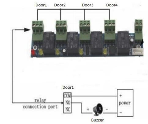
Connect the buzzer (the horn on the diagram) to the Door1 of the fire alarm bracket.
