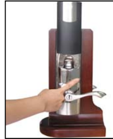
Press power button, deadbolt retracts without any users verification.
