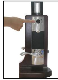
Press and hold the DEL button until number shows up, then press ↻ button to select a user ID number that you want to delete. Press the DEL button again after the user ID number was selected.
