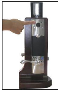
Press and hold the STOR button until "01" shows on LED display.
