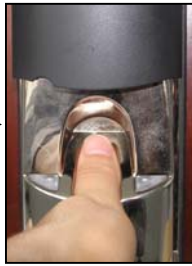
Administrator places finger on the scanner to unlock the door
