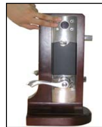
Press and hold the DEL and STOR buttons for about 5 seconds, the LED will show "UU".
